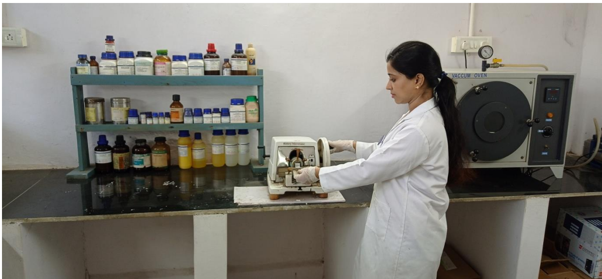
Paraffin Section Cutting on Microtome
